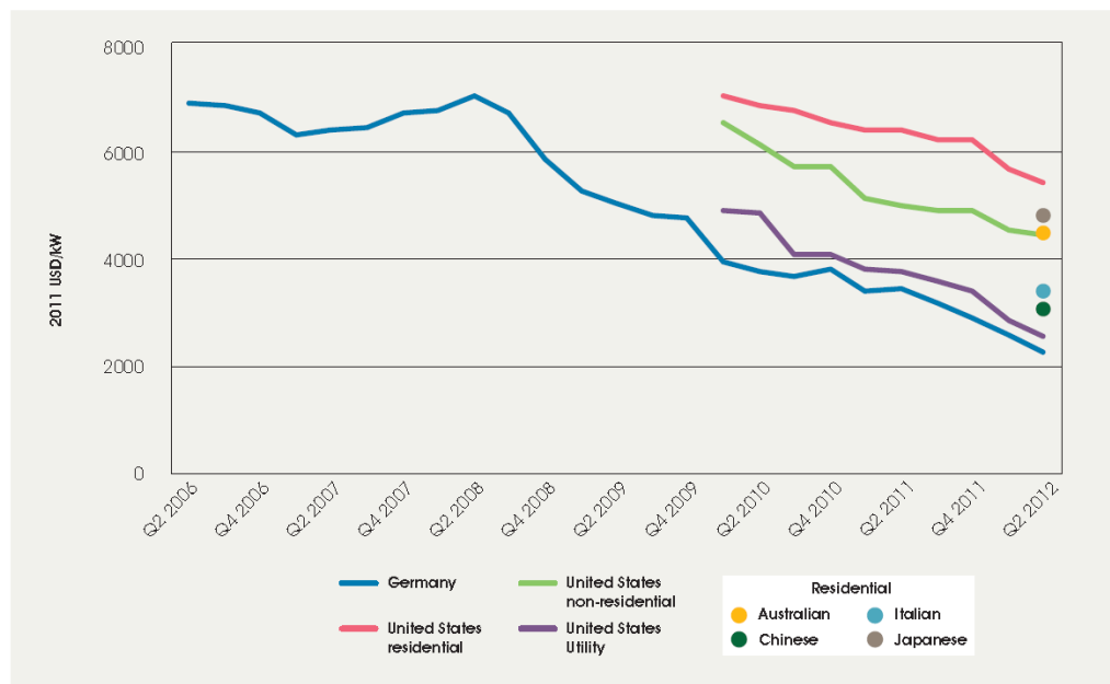
Figure A5.2 Total Installed Cost of Solar PV by Country and Sector
